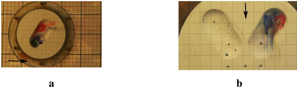
Fig. 3. Formation of stable large-scale vortex structures inside the inclined oval dimple (a) and the pair of oval dimples (b).
