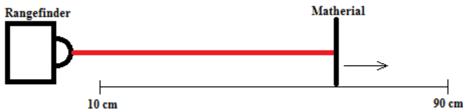
Figure 1. Geometric arrangement of the rangefinder and the studied material.
